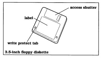
**Write-Protect Tab** - The write-protect tab is used to prevent changes being made inadvertently to important files. To write-protect a floppy, slide the write-protect tab to the open position; to allow the computer to write on the floppy, slide the tab to the closed position.
